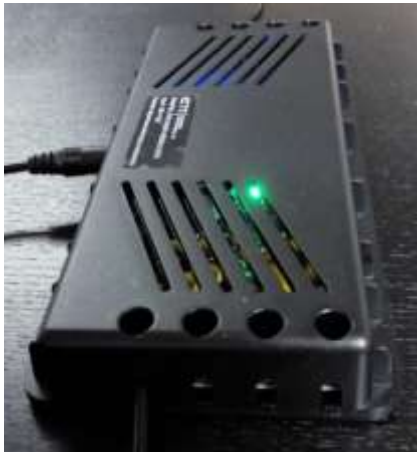
Figure 26: Green status indicator. An illuminated green LED indicates the RF Generator is operating properly and is outputting RF current
