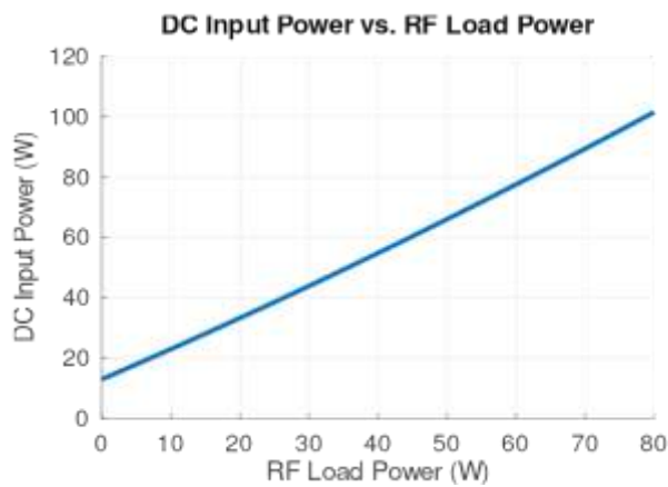
Figure 6: Test conditions: 48V, standard loop
