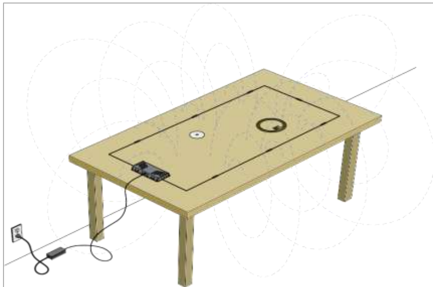
Figure 1: Magnetic field of the transmitter represented by dashed lines
