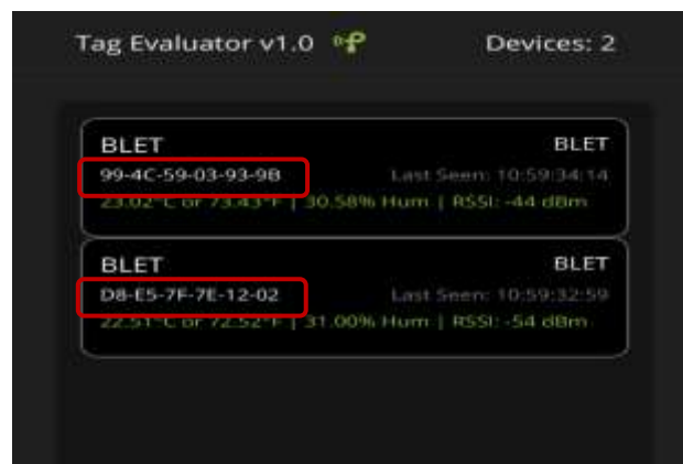
Fig 4: Two BLE Tags with the same name but different Bluetooth Device Address
